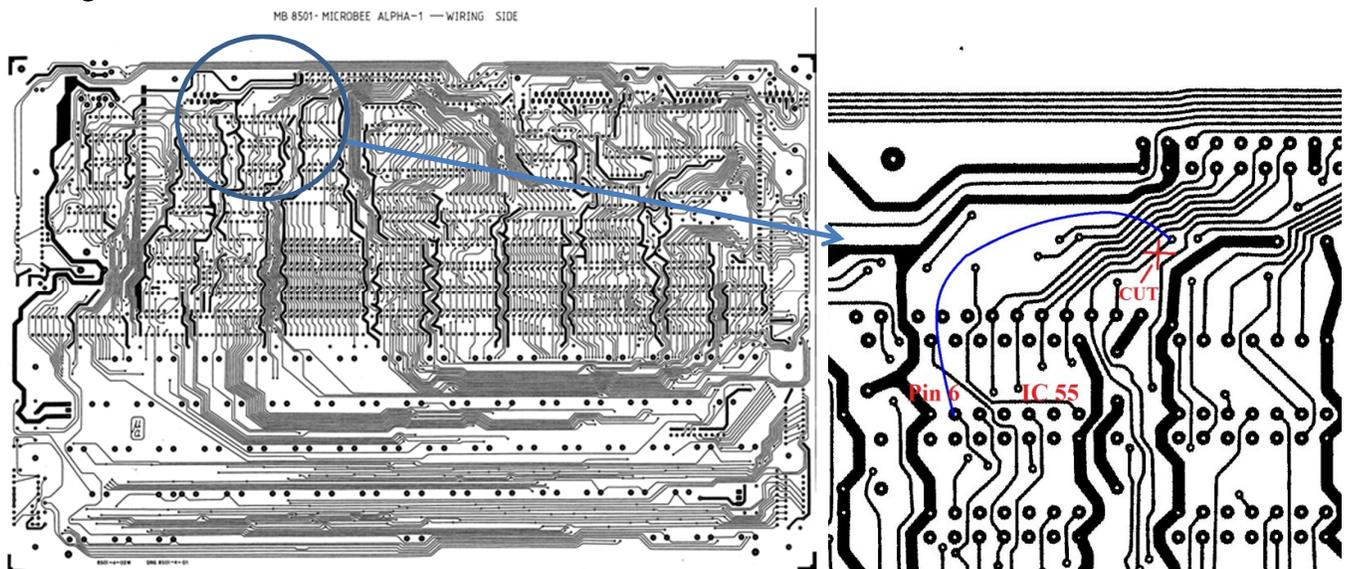
Start by cutting the track as shown in the diagram which runs from Pin 3 of RN3 to a via (drawings show underside of board where track cut is to be made). Solder a wire line (using wire wrap wire or similar) between the via of the cut track to Pin 6 of IC55.
