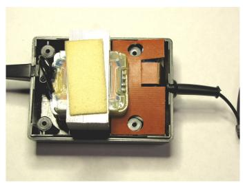
Step 4: Replace the cardboard cover & slot the strain relief grommet into the notch in the case as shown.
