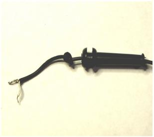
Step 1: Remove the Yellow RCA plug, strip & tin the bare ends. Place the strain relief grommet over the cable & tie a small knot in the cable as shown.
