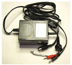
Step 5: Screw the case together. Replace the red & black RCA connectors with the red & black 3.5mm mono plugs. When finished, your plug pak supply should look like the picture above.
