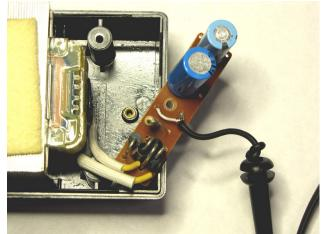
Step 2: Connect the wire to the rectifier PCB at the holes in the PCB as shown in the photo. The inner wire (the white insulated one) is the positive lead.
