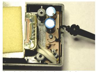
Step 3: Bolt the PCB in place with the screw & spring washer to hold it in place.
