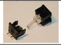
The top & bottom half of the switch are now separated revealing the plunger spring that normally sits on the plunger's round nodule & a similar node on the inside of the black key switch base.
