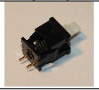
Clips either side of the switch hold the key into the key frame. Pull these out, away from the body to release the bottom from the top half of the switch.
