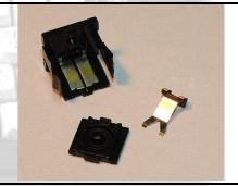
With the metal tab removed, the rubber bumper housing comes out easily & the metal switch contacts are exposed.
