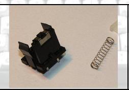
Lift the metal tab from the back of the switch to release the rubber bumper housing and gain access to the switch contacts.
