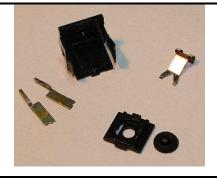
Fully disassembled switch.
