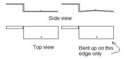
As shown in the picture, only bend the side of the contact that has the nipple in it. The left side
