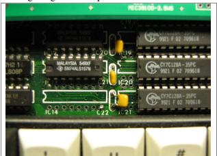
Prepare the baseboard by putting a blob of solder on both the leg of C22 nearest the keyboard, and also on pin 8 of the empty IC14 position
