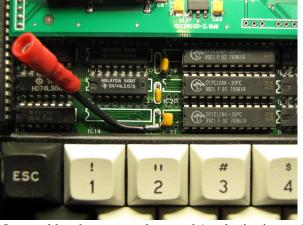
Next, solder the prepared ground 'socket' wire to the prepared points.
