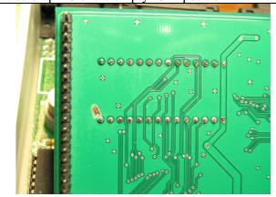
Next, scrape away some of the solder mask near pin 14 of the Eprom socket on the coreboard.
