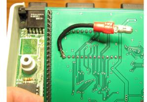
Attach the prepared ground 'plug' to the exposed copper and also pin 14.
