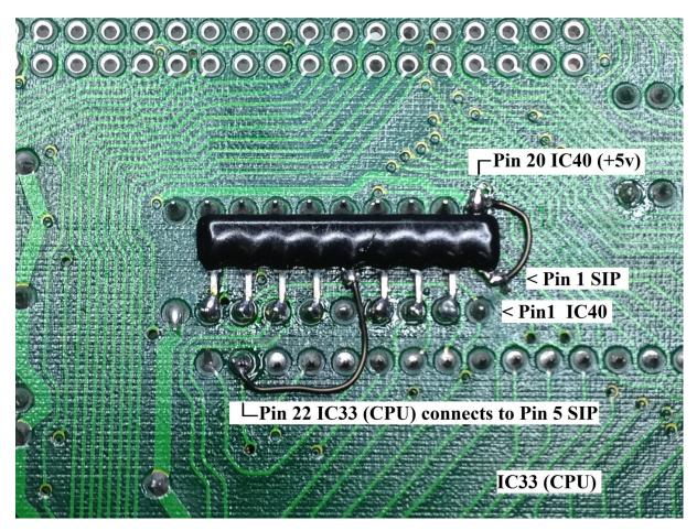
There are no track cuts to be done, so once fitting is completed as per the above photo, re-assemble & test the Microbee.
